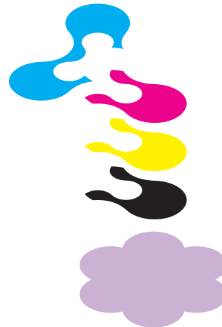
Applying the Difference blending mode produces five color plates because flattening requires conversion of the spot into process colors to properly blend the colors.
